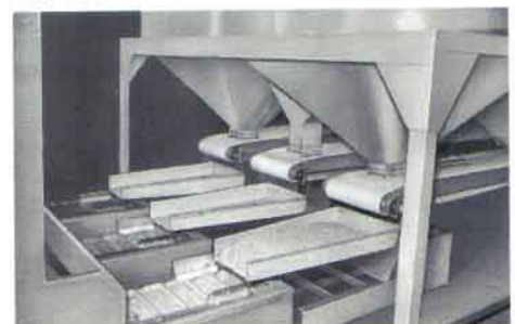
Withdrawal system from storage bins, belt conveyors, vibratory conveyors and bucket elevators shown.
